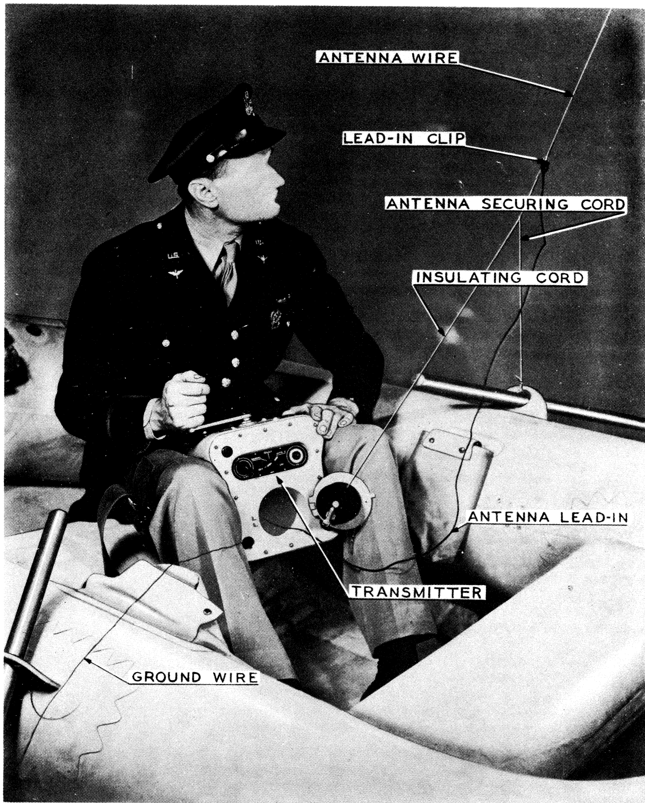
Figure 20—Radio Transmitter BC-778-E in Operating Position
